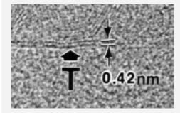
**Q**Hi-res image Electron microscopic examination of carbon nanotubes (indicated by arrows).
